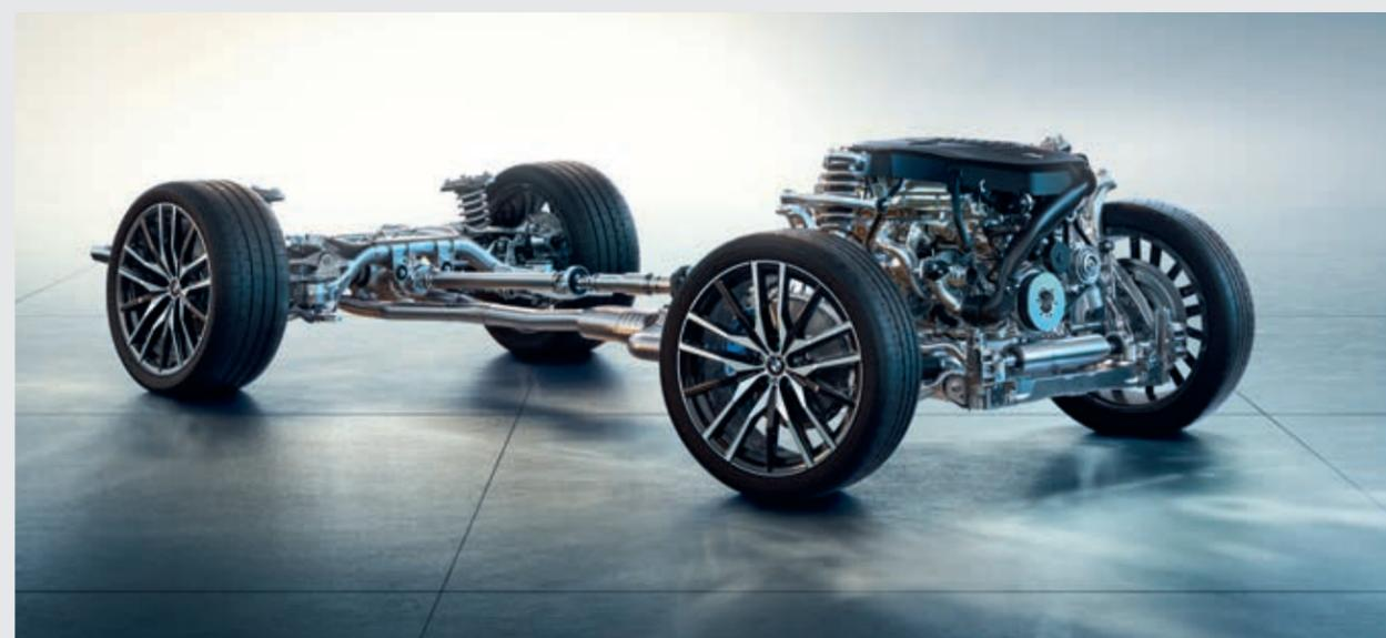
The Adaptive 2-axle Air Suspension makes driving particularly comfortable with high driving dynamics and makes it easier to get in and out and load the vehicle. The air suspension automatically keeps the vehicle at a constant height regardless of the load. It can also be raised or lowered manually at the touch of a button.
