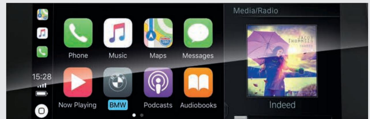
Preparation for **Apple CarPlay**<sup>1,2</sup> supports the convenient and wireless use of selected iPhone® functions in the vehicle. This allows smartphone content and functions such as music, iMessages/text messages, telephony, Siri and selected third-party apps to be displayed and operated via the vehicle's user interface and via voice control.
