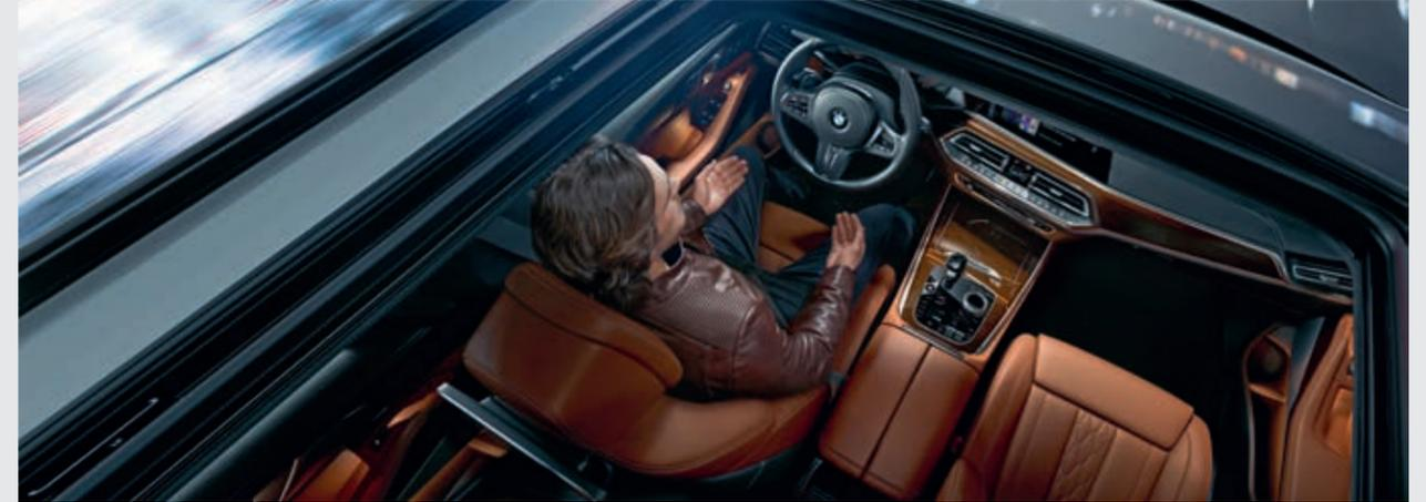
When open, the **Panorama Glass Roof** provides a great deal of fresh air. And when closed, it creates a bright, light-flooded atmosphere in the interior. It opens and closes completely automatically at the push of a button, and is equipped with slide and lift functions, roller sunblind and wind deflector.
