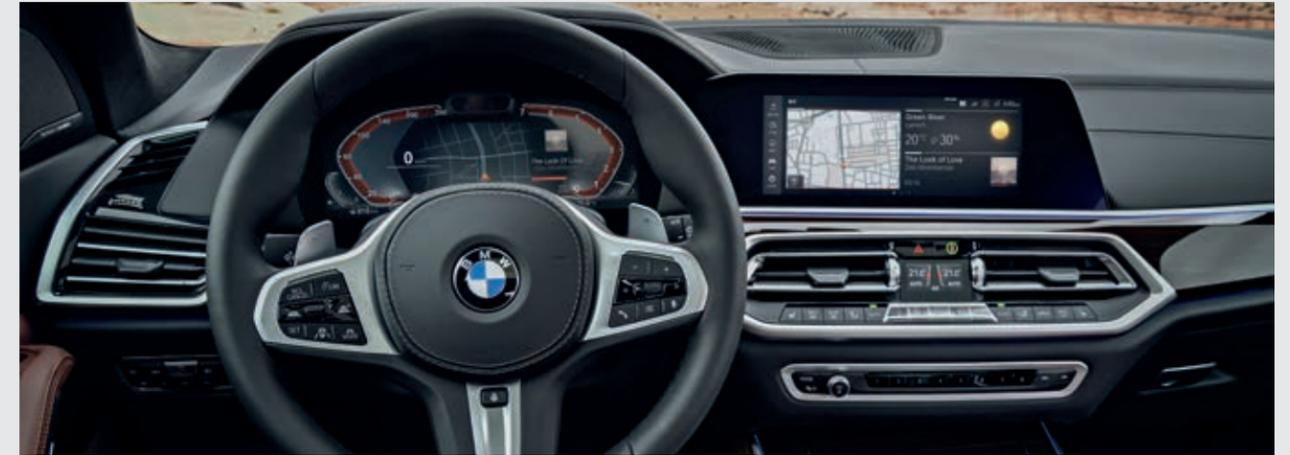
The **BMW Live Cockpit Professional** with navigation function includes a high-quality display network consisting of a high-resolution 31.2 cm (12.3 inches) Info Display that can be operated by touch and a fully digital 31.2 cm (12.3 inches) instrument cluster.
