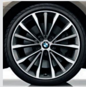
19" light alloy V-spoke style 663 I wheels bi-colour, front 8J x 19 with 245/40 R19 tyres and rear 9J x 19 with 275/35 R19 tyres.
