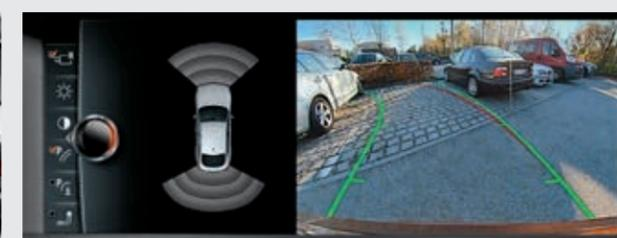
The **Reversing Assist Camera** enables improved orientation when reversing at speeds below 10 kmph. It shows the area behind the car on the Control Display. Interactive track lines for measuring distance and turning circles assist the driver when manoeuvring, obstacles are marked in colour.
