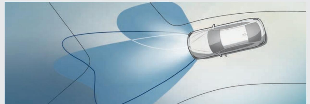
**LED Headlights with Adaptive headlights**, variable city and motorway light distribution and BMW Selective Beam provide optimum illumination of the road when driving in the dark. Even at a standstill, the integrated cornering lights are automatically activated by signalling or turning the steering wheel and are active at speeds of up to 35 km/h.
