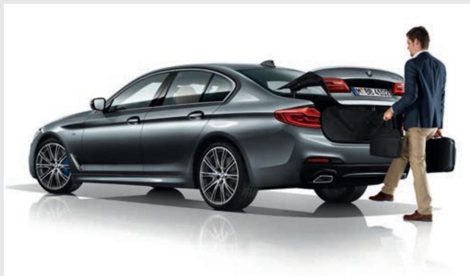
The **Comfort Access** with smart-opener makes it possible to open all four vehicle doors, including the luggage compartment, without using the key. This equipment includes contactless opening of the bootlid with a quick wave of the foot under the rear bumper.
