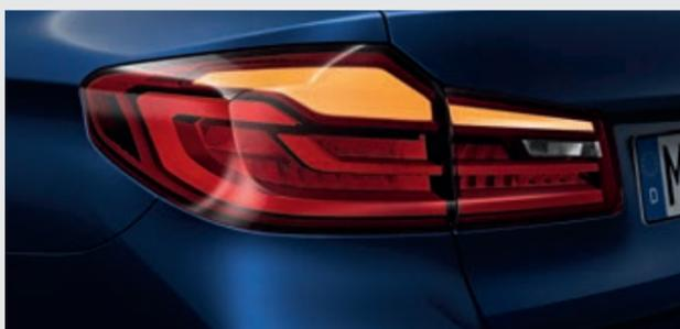
The **LED Rear Lights** are split into two parts, with LED technology featured in the tail lights, brake lights, turn indicators and reversing lights.
