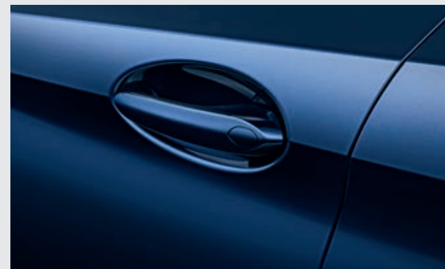
Effortless and quiet: soft close automatic ensures that the doors are securely closed with a minimum of exertion and without unpleasant noise.
