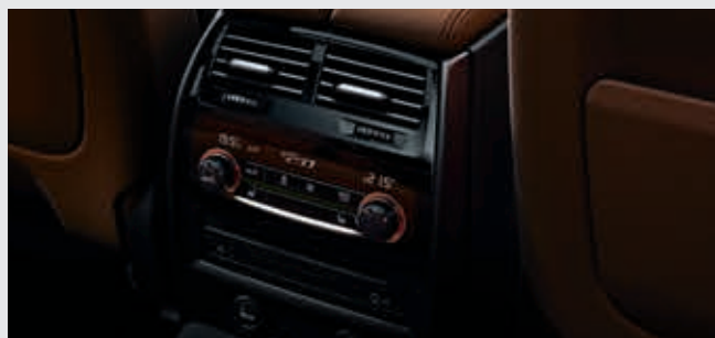
The automatic air conditioning with 4-zone control comes with the equipment included in Automatic air conditioning with 2-zone control with extended contents, along with two air vents in the B columns.
