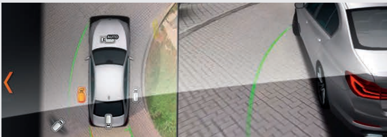
Parking Assistant with Surround View Camera makes parking and manoeuvring the vehicle easier. The Parking Assistant with linear guidance parks the vehicle automatically, parallel or perpendicular to the street. Surround View includes the camera-based functions like Rear View Camera, Panorama View, Top View and 3D View. The cameras in the exterior mirrors as well as at the front and rear of the vehicle allow for a 360° all-around view.
