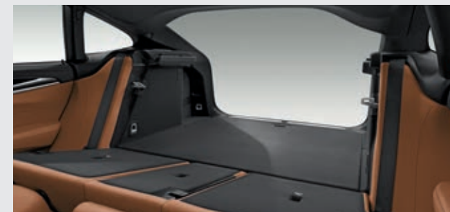
The Through-loading system consists of rear seat backrests that are divided in a 40:20:40 ratio, guaranteeing more flexibility when transporting people and objects. For example, two passengers can be seated comfortably in the rear, while long objects such as ski and snowboard bags can be transported at the same time.
