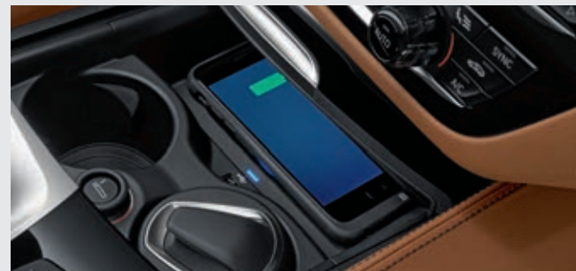
Telephony with wireless charging 1 includes a wireless charging dock and additional USB ports. A roof aerial connection improves mobile reception. Two mobile telephones and an audio player can be connected simultaneously via Bluetooth.
