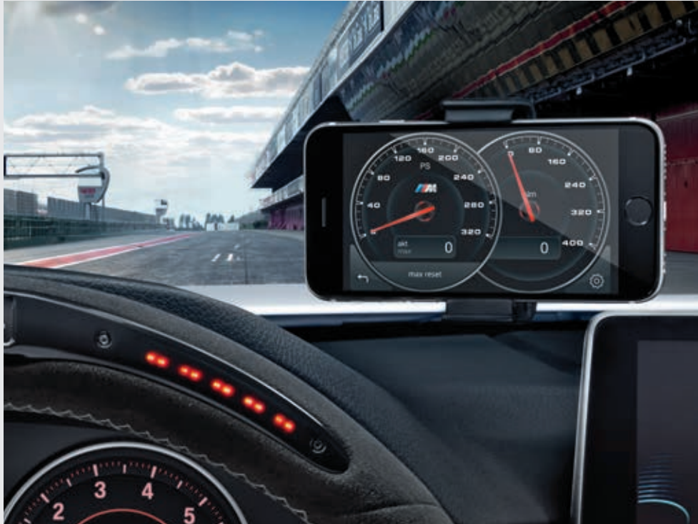
M Performance Drive Analyser. The Drive Analyser comprises of an on-board diagnostics stick and a smartphone app to collect and analyse a variety of technical driving data.
