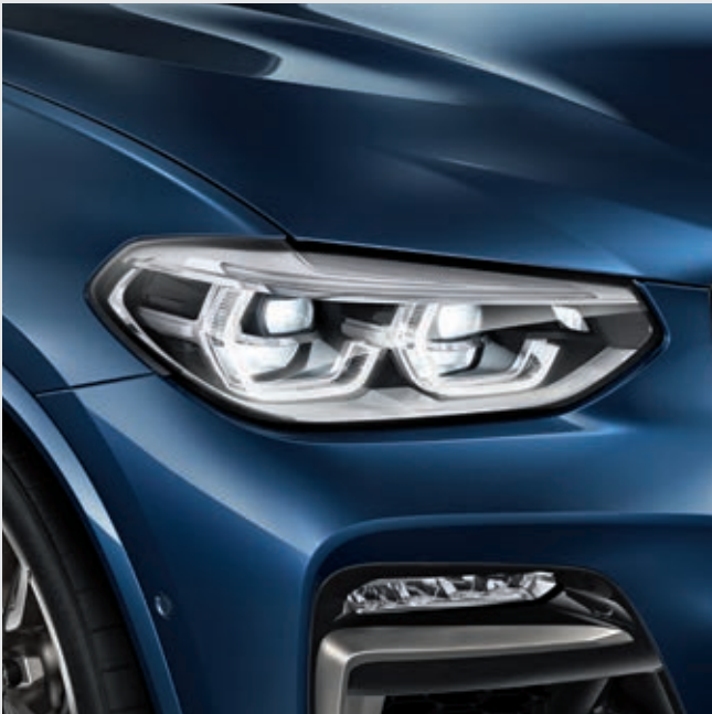
The Adaptive LED headlights include low-beam and high-beam headlights and turn indicators with full LED technology. The equipment also features BMW Selective Beam, cornering lights, daytime running lights and Adaptive headlights with variable light control for excellent illumination of the road ahead and better visibility in the dark.
