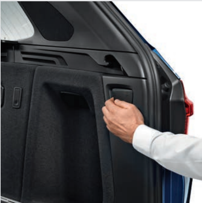
Remote backrest unlocking for the rear seats allows the rear seat backrests to be unlocked and folded down conveniently via a button in the luggage compartment.
