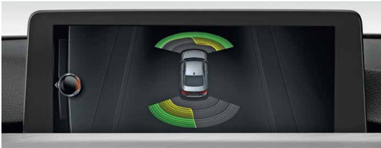
The Park Distance Control (PDC), front and rear allows for easy parking and manoeuvring in confined spaces. Acoustic signals and a visual indicator in the Control Display tell you when the front or rear of the vehicle is approaching an object. Distances are measured by ultrasound sensors in the bumper.
