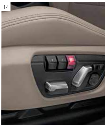
[ 12 ] Door sill finishers in aluminium with "BMW" designation. [ 13 ] 22.3 cm (8.8") LCD colour display with touch functionality and configurable user interface. [ 14 ] Memory function on front seats enables you to save your settings for the position of the seat, backrest, steering column and exterior mirrors.
