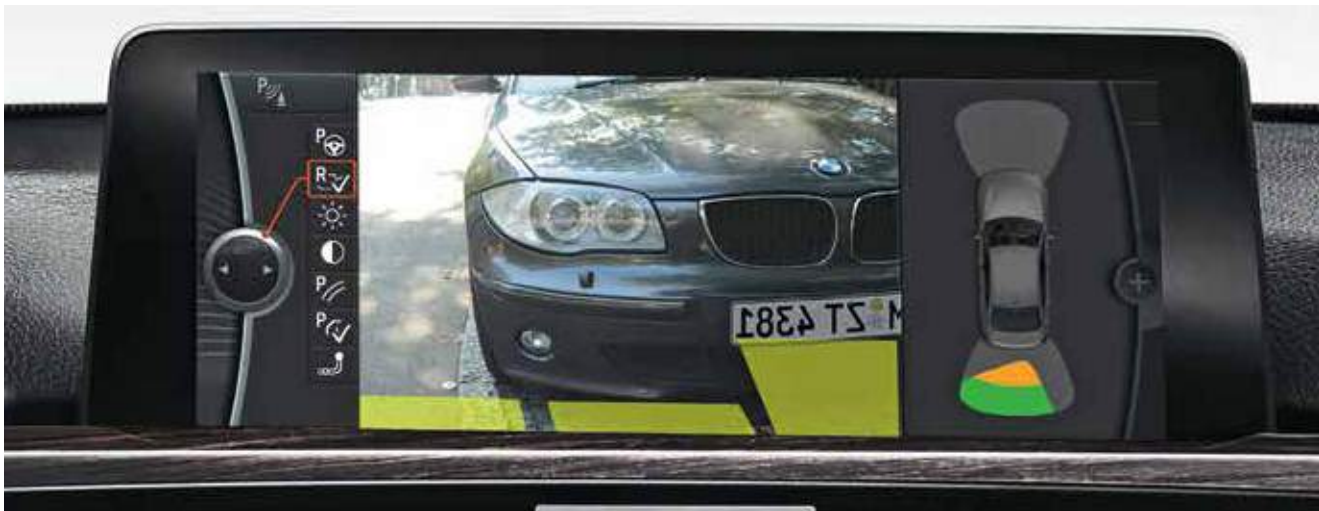
The Rear-View Camera allows you to view the area behind the car in the Control Display while manoeuvring and parking. The Rear-View Camera enhances visibility when reversing at speeds below 20 km/h.
