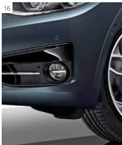
[ 15 ] Automatic tailgate operation allows users to open and close the tailgate electronically at the push of a button. [ 16 ] LED fog lights increase short-range visibility in fog or precipitation, improving night-time driving safety. [ 17 ] Active rear spoiler optimises the air flow at the rear of the car as your speed increases, to ensure excellent road holding.
