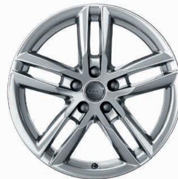
Audi Sport cast aluminium alloy wheels, 5 twin-spoke design size 7J x 18, with 235/50 R18 tyres
